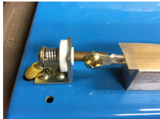
Figure 7. Loosen screw on front spring hook
