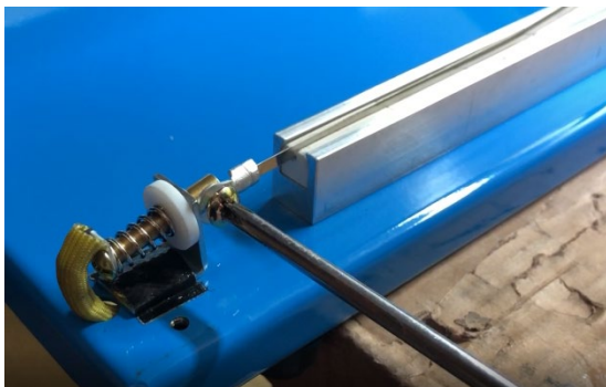
Figure 8. Connect heating element to front spring hook.
